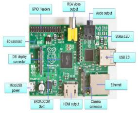
Fig2.Raspberry Pi model B
